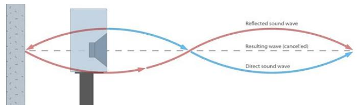
The other thing that happens, when a loudspeaker is moved to a boundary is, that the sound reflected at the boundary will come back to the listener, but now with a latency, compared to the original (non-reflected) sound.
