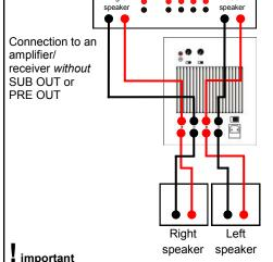
Amplifier/receiver and the subwoofer must be turned off while the connection is being made.
